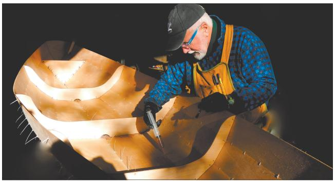
Marty Loken works to assemble a small wooden boat using stitch-and-glue construction. Photo courtesy Marty Loken
