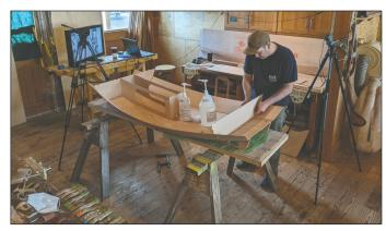
Liam Crist-Dwyer assembles a small boat called a "Portage Pram" using the glue-and-stitch construction method. Photo courtesy of Northwest Maritime Center
